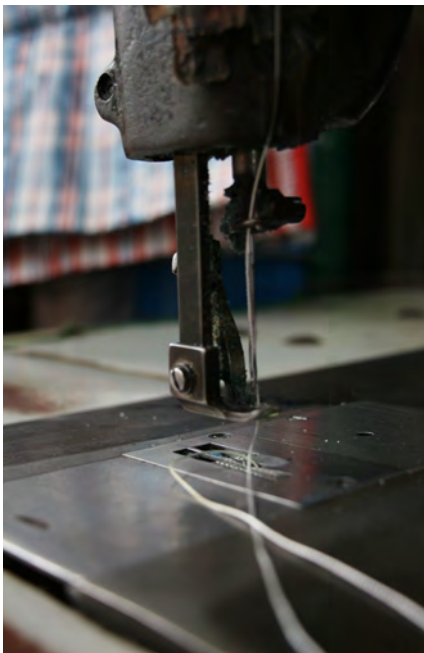
Canvas are sewn with a normal nylon thread and a thick intertwined nylon thread for better durability of the final product.
