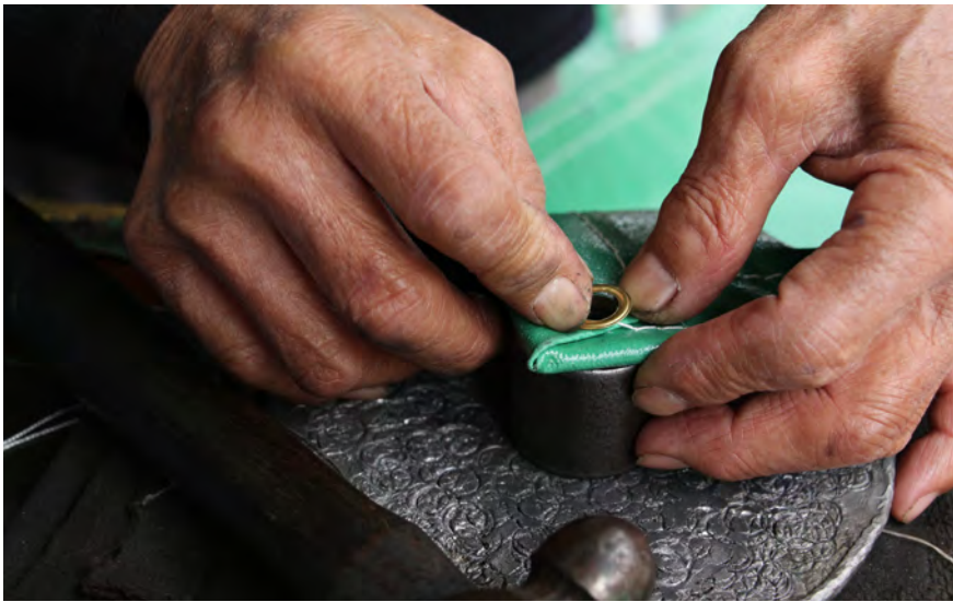
The top of a flat ring will be placed on one side of the canvas and it will be hammered to the bottom of the ring on the other side.
