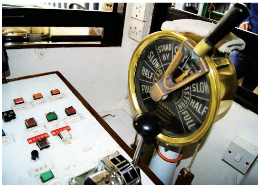
A chadburn is a clock-like device with different orders about engine speeds.
