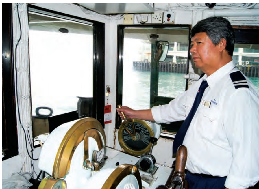
Star Ferry captains order the chief engineer in the engine room by pulling the handle of the chadburn.
